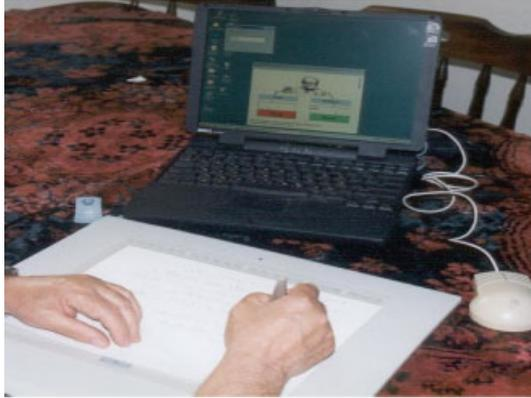
Figure 1. The computerized system, including laptop computer, ComPET software, and digitizing tablet.
